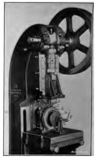
Fig. 2. Perforating Attachment with Special Device for Holding Shell in Place
